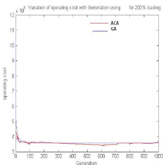
Figure 7. Variation of Total Cost with Generation for 200 % Reactive loading
